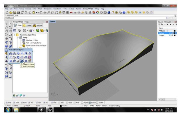
**Step 5** Convert the generated UV Curve to a Planar Surface with the "PlanarSrf" command.
