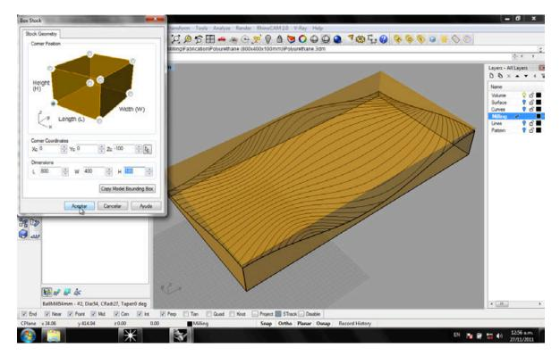
Create an engraving pattern, in the 2-1/2 Axis menu. Set the tool to the 54mm ball.
