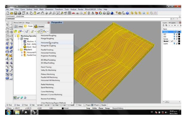
Set the tool to the 26mm ball and press generate.
