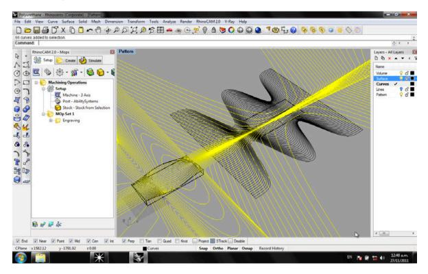
Split the lines in order to clean the pattern to be milled onto the model surface.
