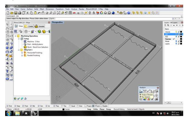
Create a tight loft surface with 50 control points with the curves.
