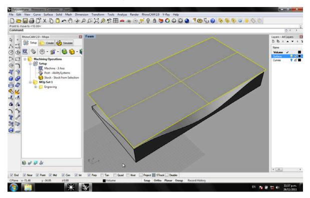
Take the surface out of the model area, to make it easier to design the milling pattern.
