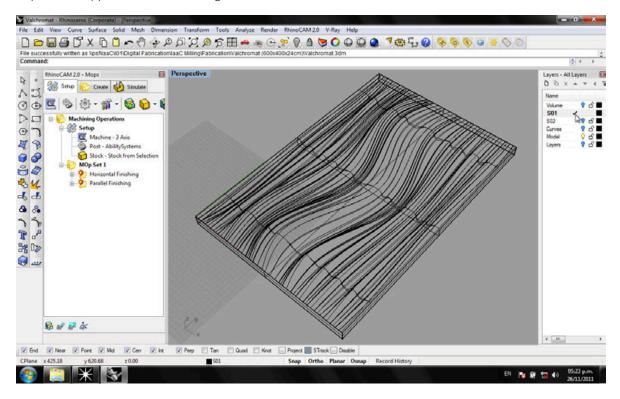
Copy the model in a new layer and cut it in three 12mm layers using the split tool in the frontal view.
