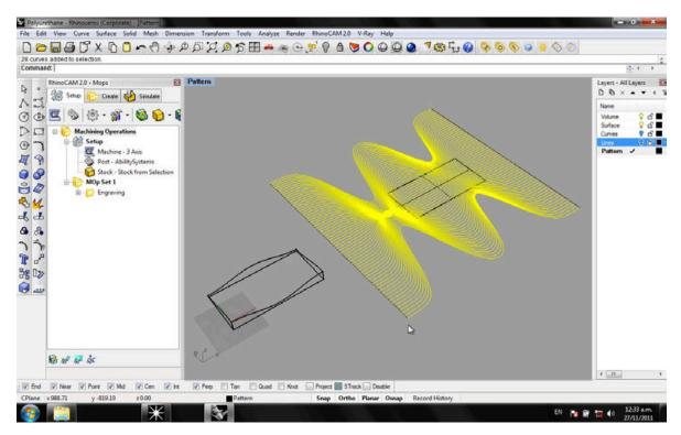
Run the "FlowAlongSrf" command and select all the lines, then, select the base surface.
