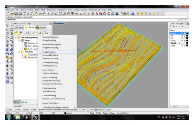
Set the tool to the 6mm ball and press generate.
