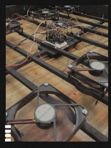
Fan Power 12v 0.28A Fan Current Fan Dimension 15cm Arduino 01 Cables 2m Light sensors 04
