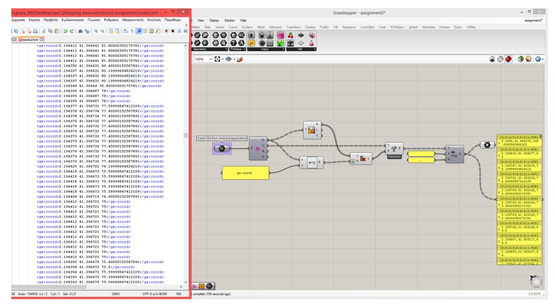
Process the data from tracks1.kml by isolating only the coordinates of the points.
