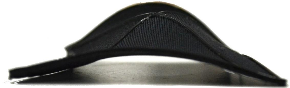
Sample deformation by 3d-printing on fabric
