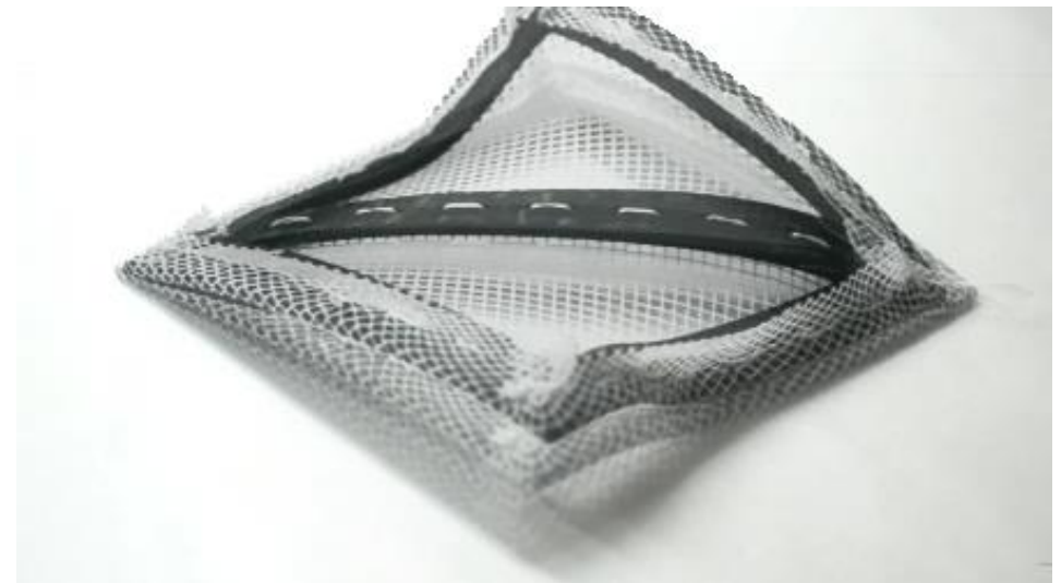
Sample deformation by adjusting shape memory polymer on fabric
