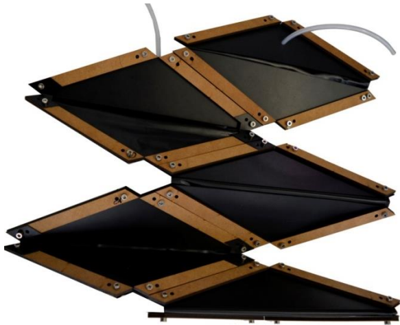
State: Inflated Expansion: >75% Pressure: <1 psi
