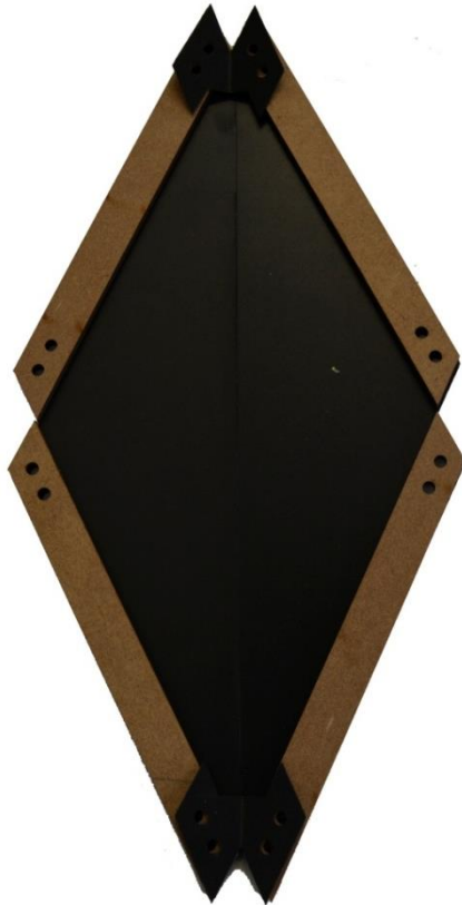
Frame pocket and joints Material: PVC Thickness: 2mm Density: 1.1 – 1.45 g/cm3
